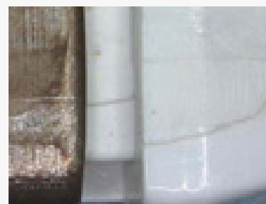
Linear cutter, cracked, holding blood & skin tissue
